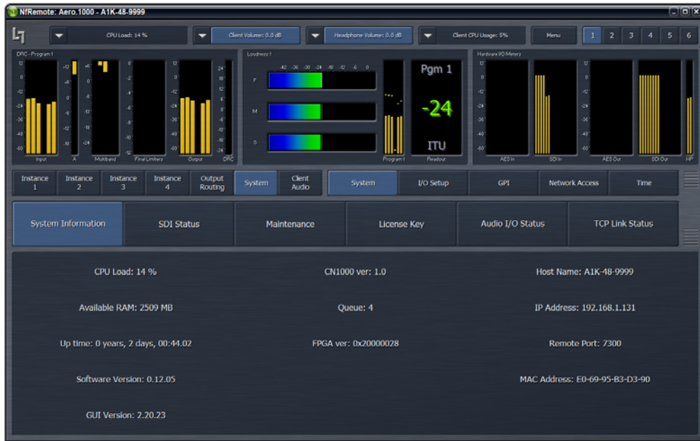
Figure 1-11 IP address, remote port, MAC address, and other system information
