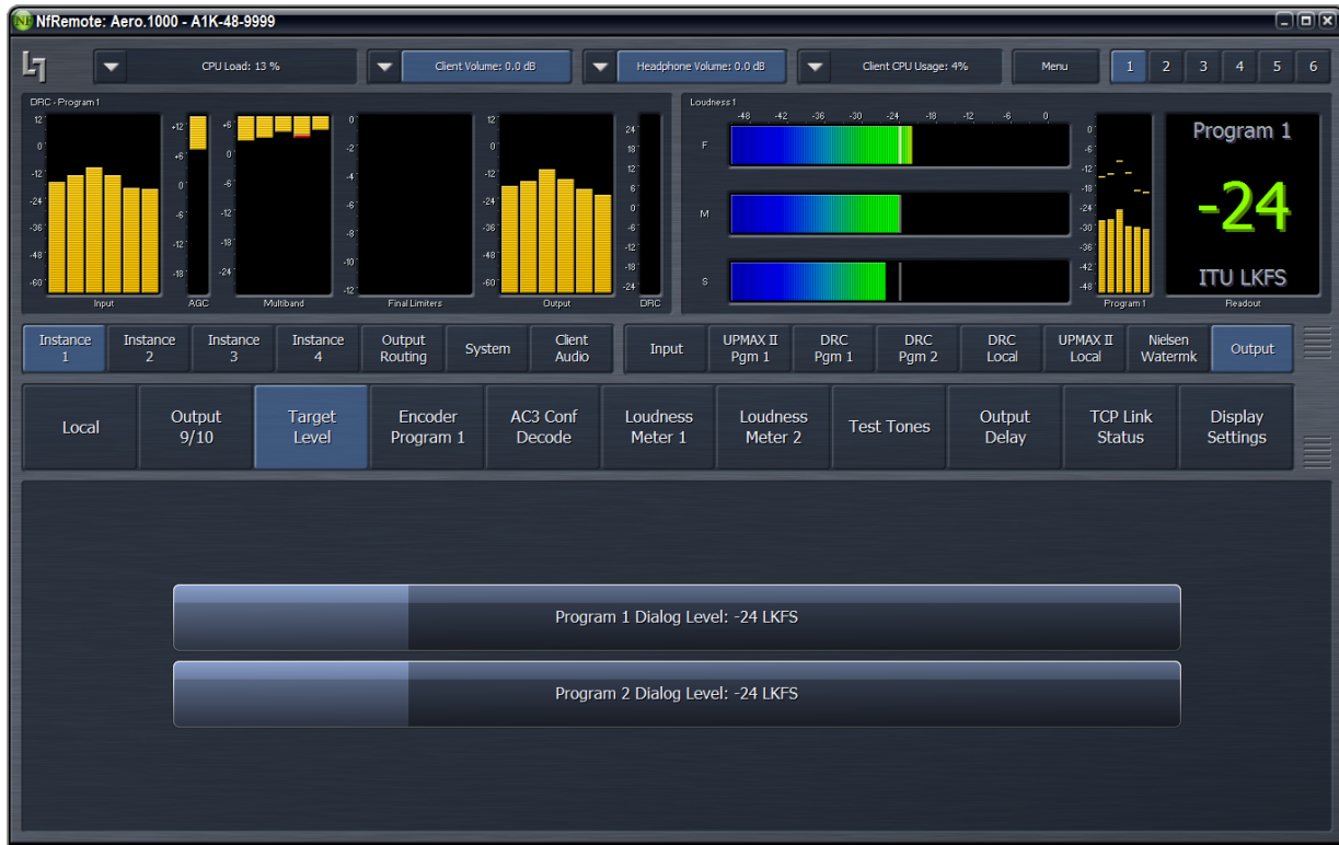
Figure 1-21 Adjusting the target level (dialnorm) to match the meter
