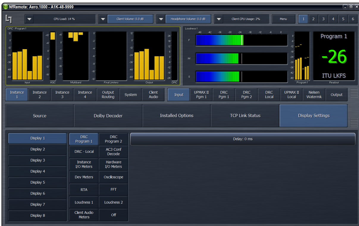
Figure 2-7 Display Settings menu in lower section
