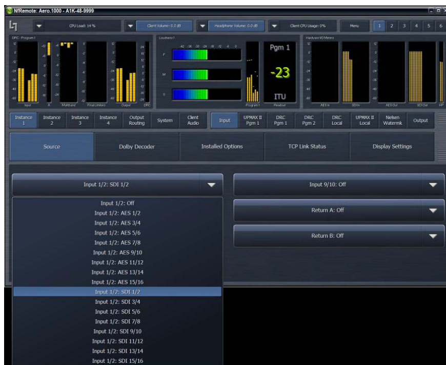
Figure 1-8 Drop-down menu for each Instance input lists all physical inputs
