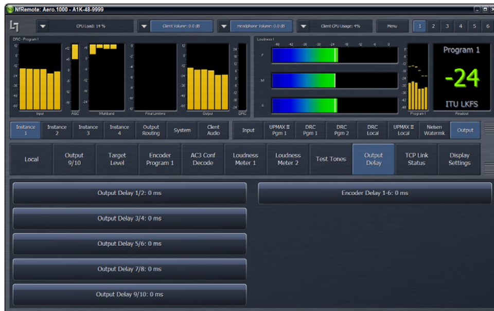
Figure 1-14 Output Delay settings available for each instance
