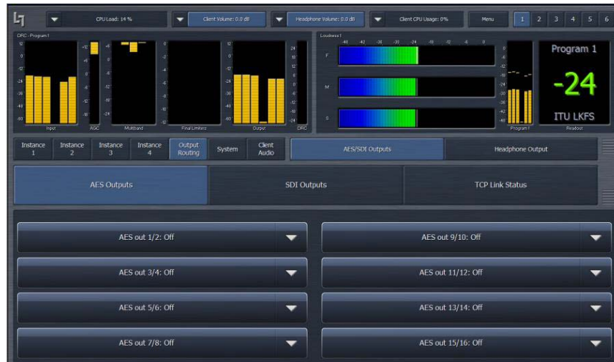
Figure 1-9 The AES and SDI Outputs tabs allow source selection for each physical output
