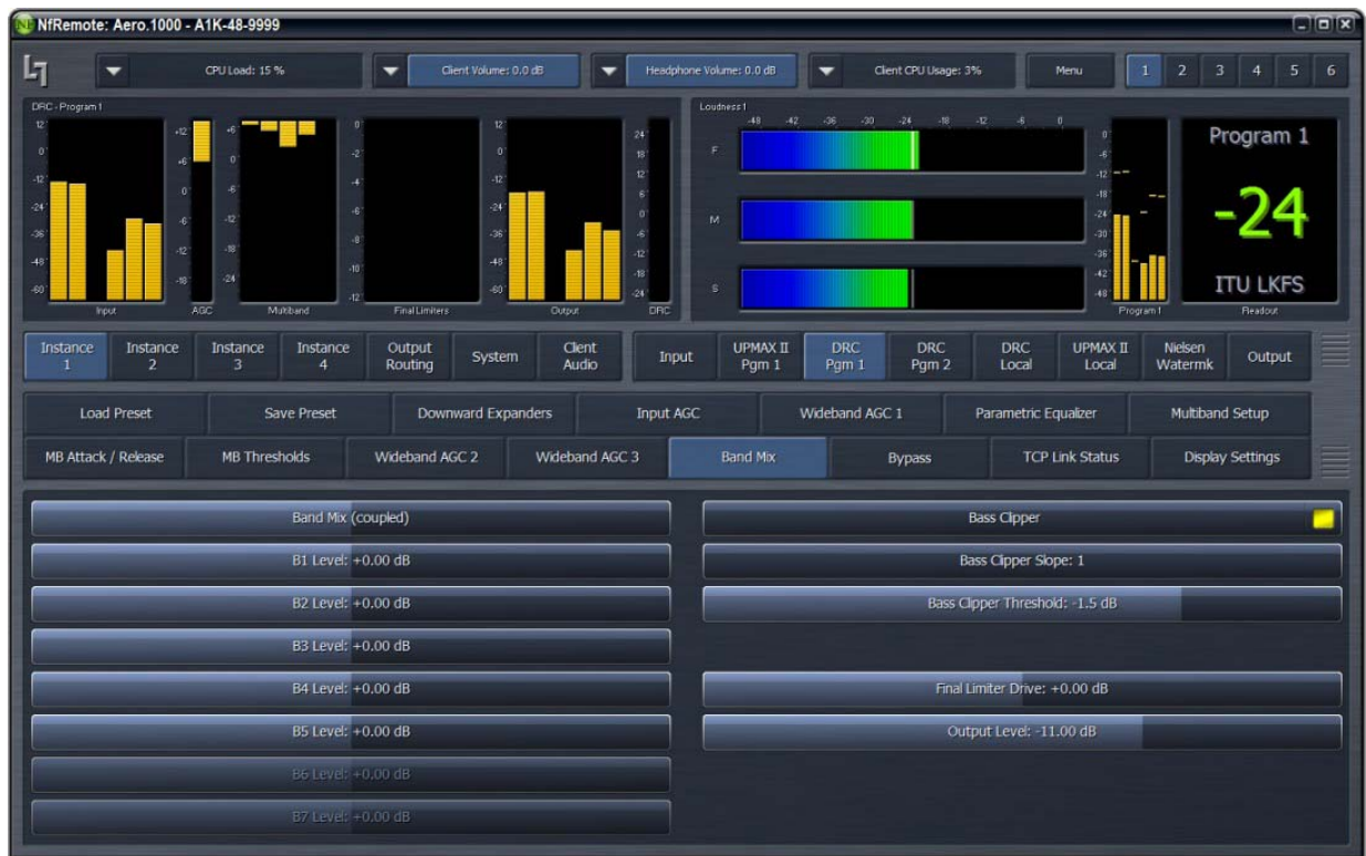
Figure 1-20 Adjusting Output Level so the meter matches the target
