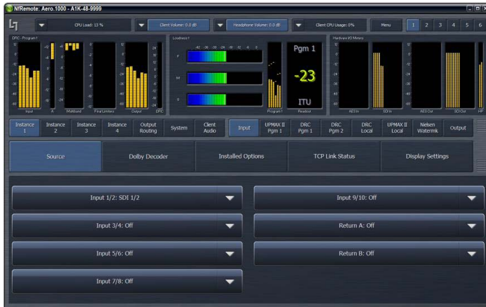
Figure 1-7 Available inputs for 5.1+2+Local instance: 1–6 + 7–8 + 9–10
