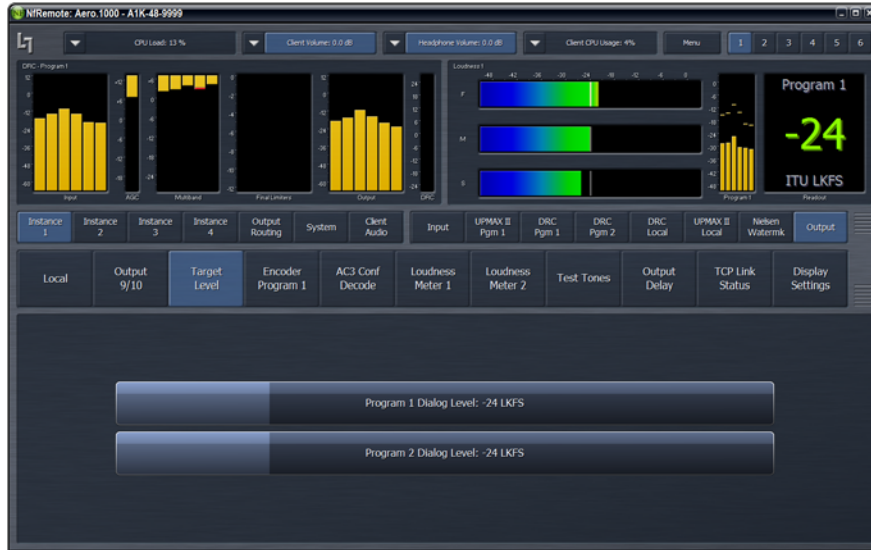
Figure 1-18 Dialog level (dialnorm) is set under the Target Level tab
