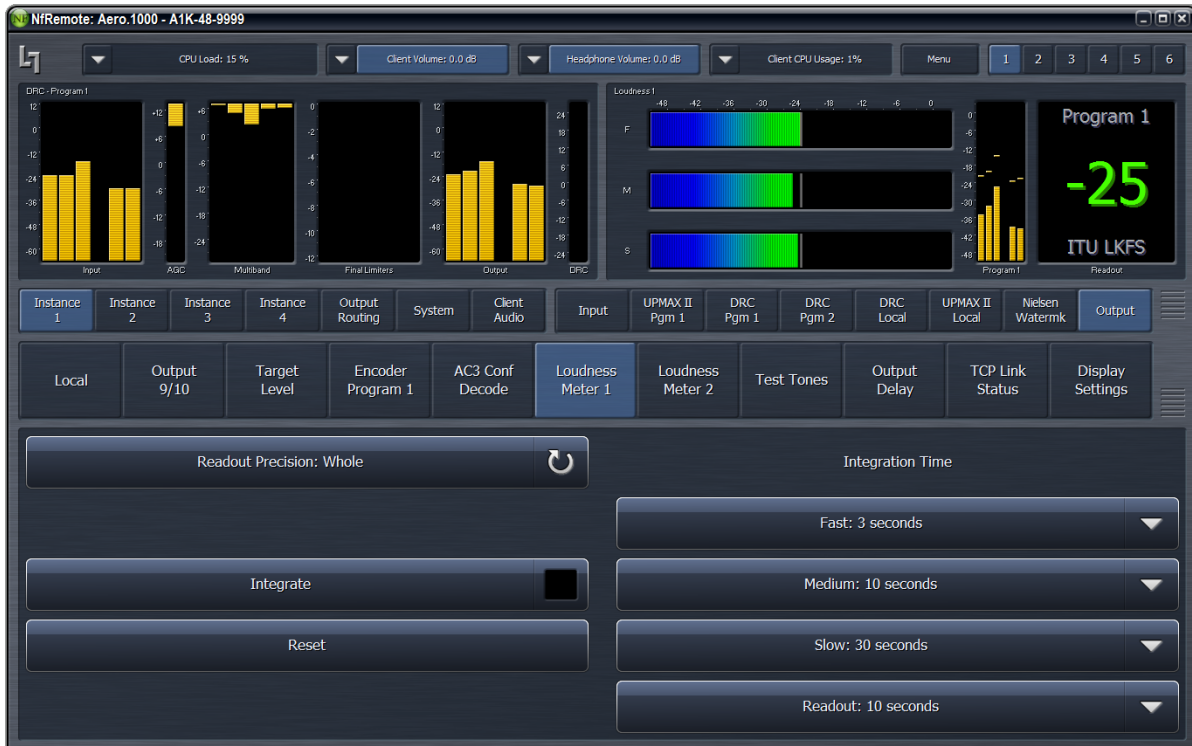
Figure 2-9 Settings for the program-specific ITU meter
